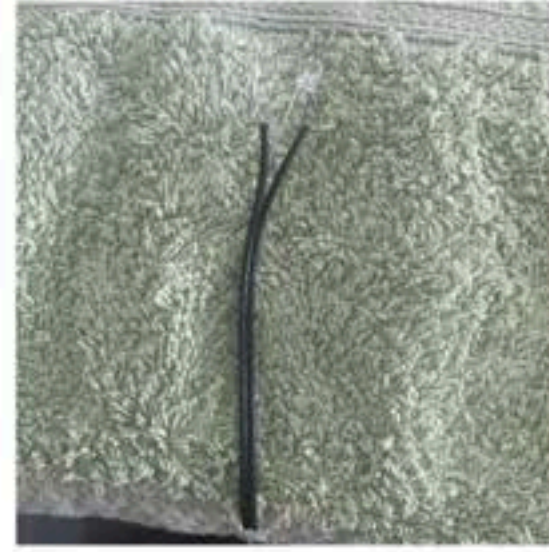
CUT BLACK EXTERIOR OF THE WIRE TO EXPOSE IT + ATTACH TO LED LIGHT
