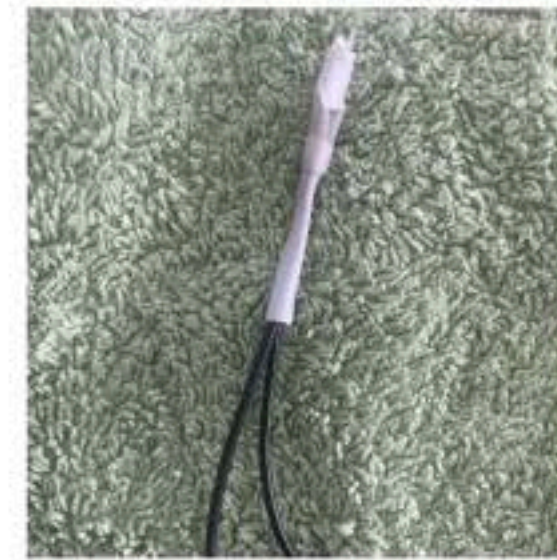
BURN THE TUBING TO MELT IT DOWN + SECURE
